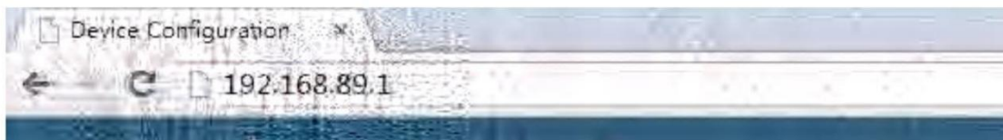
Figure 3-2-2 enter into Web configuration through LAN port
